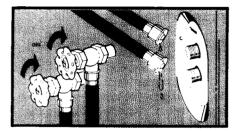
1. Shut off both water faucets. Disconnect and drain water inlet hoses.
